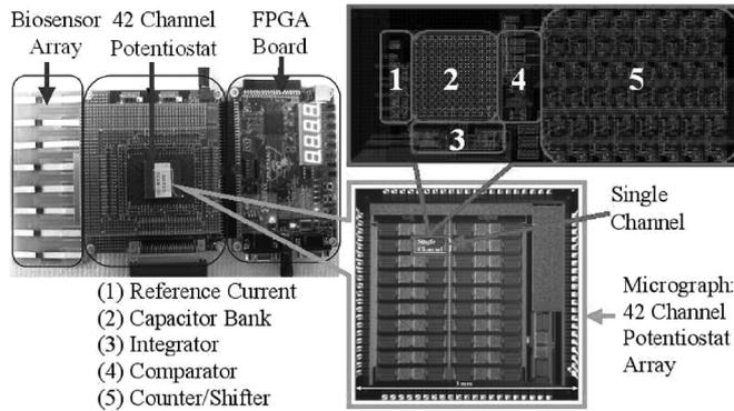
Fig. 9. Experimental setup showing the interface between biosensor array with the multichannel potentiostat.
