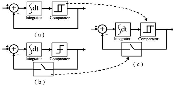
Fig. 1. Architecture of (a) time-encoded modulation (TEM) (b) continuous time  $\Sigma\Delta$  (c) semi-synchronous  $\Sigma\Delta$  converter.
