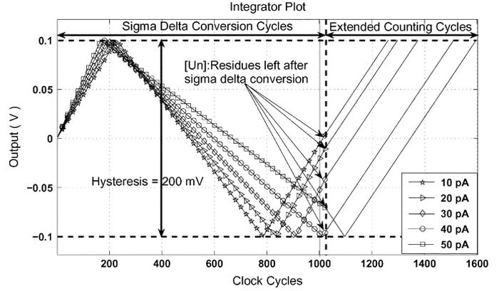
Fig. 4. Illustration of compensation step for the semi-synchronous  $\Sigma\Delta$  conversion. The residue at the end of synchronous conversion is discharged (charged) using a reference current to a reference potential  $\Delta$ .
