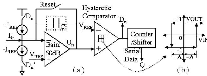
Fig. 2. Architecture of the proposed semi-synchronous  $\Sigma\Delta$  converter.  $D'_n$  denotes the complement of  $D_n$ .
