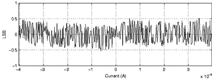
Fig. 6. Measured DNL plot for a semi-synchronous  $\Sigma\Delta$  converter.
