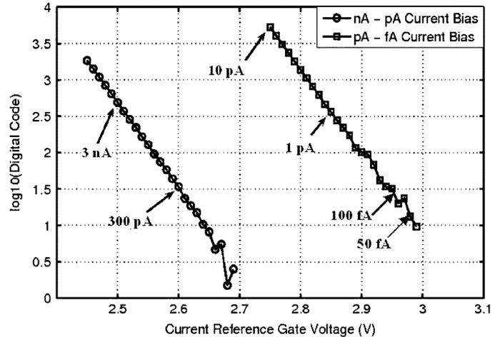
Fig. 7. Demonstration of the potentiostat for measurement of subthreshold characteristics of a pMOS transistor, whose drain current can be as low as 50 fA.
