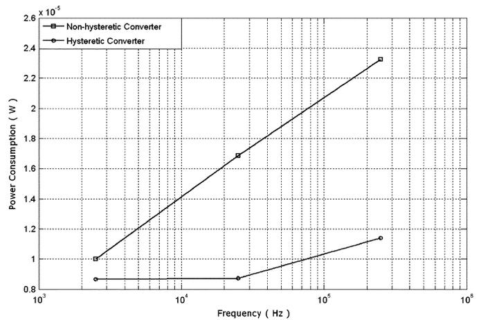
Fig. 8. Comparison of power dissipated by a semi-synchronous  $\Sigma\Delta$  with a conventional  $\Sigma\Delta$  for different sampling frequency.
