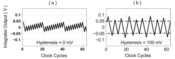
Fig. 3. Comparison of integrator output at different hysteresis levels (a) 0 V and (b) 100 mV.
