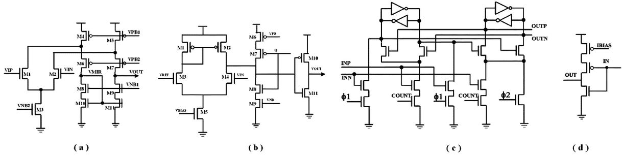
Fig. 5. (a) Folded cascode op-amp used for implementing the integrator. (b) Schematic diagram of hysteretic comparator. (c) Schematic of the counter/shift register cell. (d) Current starved inverter used in counter/shift register.
