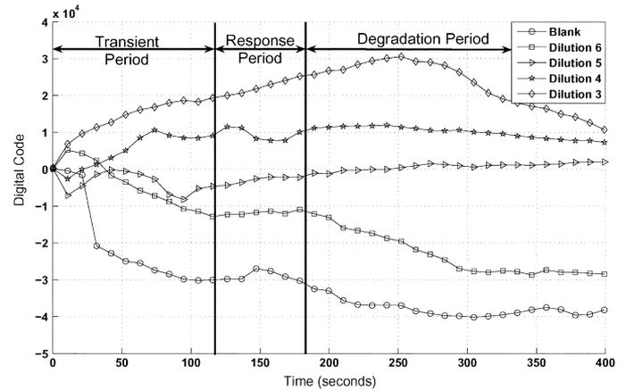
Fig. 10. Measured response of a *Bacillus Cereus* biosensor for different concentration levels Dilution 6:  $10^6$  CFU/ml, Dilution 5:  $10^5$  CFU/ml, Dilution 4:  $10^4$  CFU/ml, Dilution 3:  $10^3$  CFU/ml, Control Solution: Blank.
