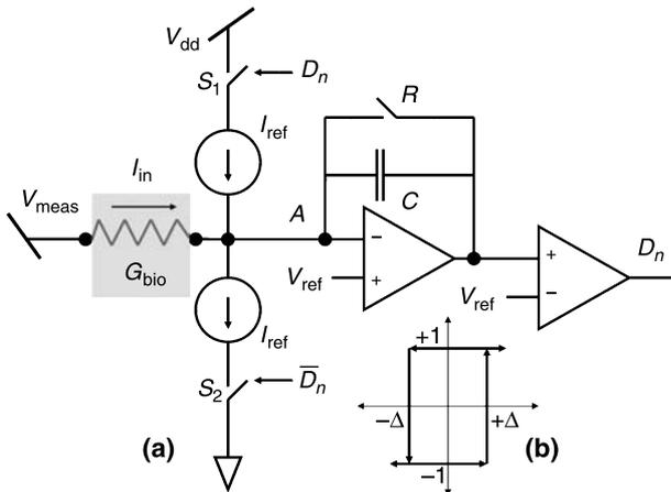
**Fig. 4.** Architecture of a semi-synchronous  $\Sigma\Delta$  modulator which interfaces with the immunosensor (represented by a conductance)
