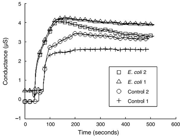
**Fig. 9.** Conductance measured across two antibody capture zones (marked by 1, 2) when an analyte containing *E. coli* is applied
