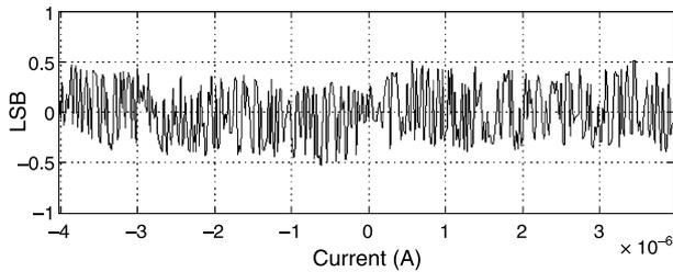
**Fig. 6.** Measured DNL plot for a semi-synchronous  $\Sigma\Delta$  converter
