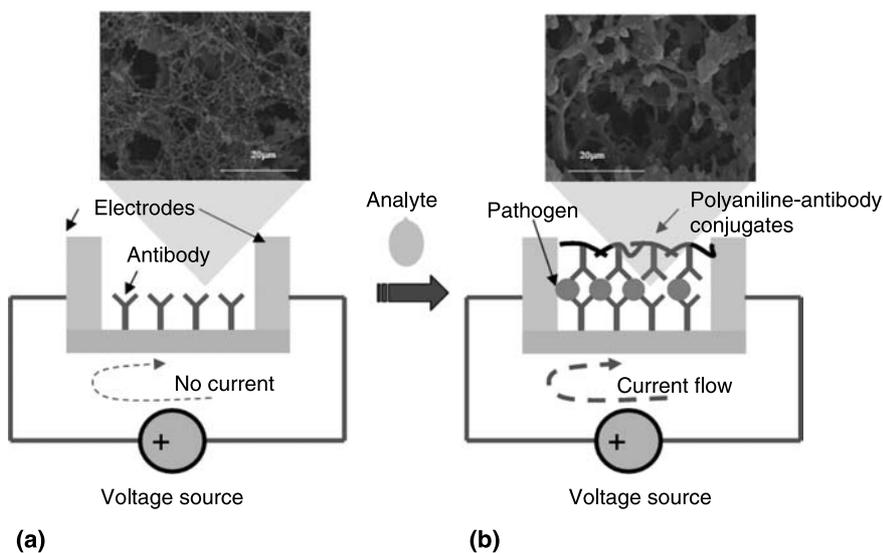
**Fig. 2.** Principle of operation of the biosensor with illustration of the two states by SEM images
