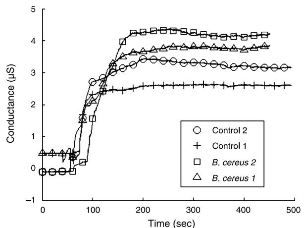
**Fig. 8.** Conductance measured across two antibody capture zones (marked by 1, 2) when an analyte containing *B. cereus* is applied
