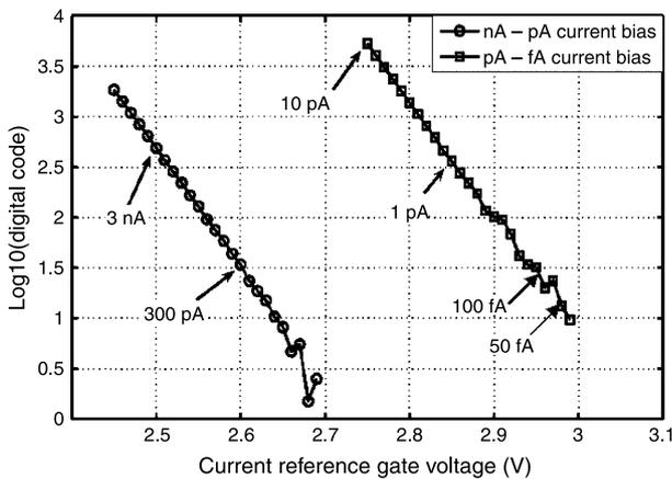
**Fig. 7.** Demonstration of the potentiostat for measurement of sub-threshold characteristics of a p-MOS transistor, whose drain current can be as low as fA
