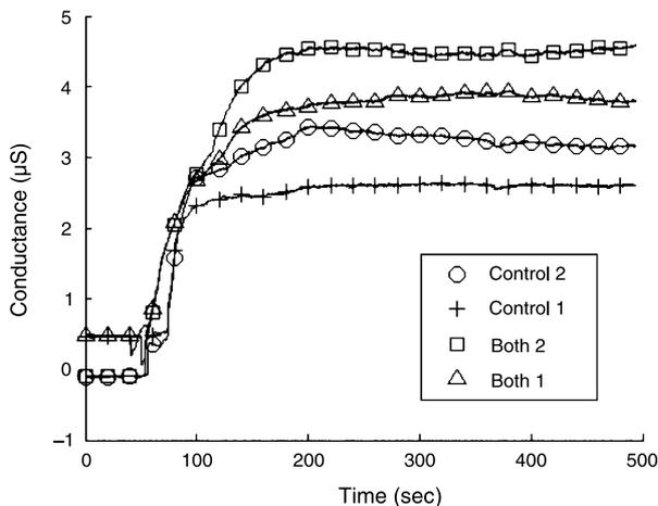
**Fig. 10.** Change in conductance across two antibody capture zones (marked by 1, 2) when both pathogens (*B. cereus*, *E. coli*) are present
