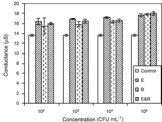
**Fig. 11.** Change in conductance across the mixed antibody biosensor for different concentration of pathogens (*B. cereus*, *E. coli*)
