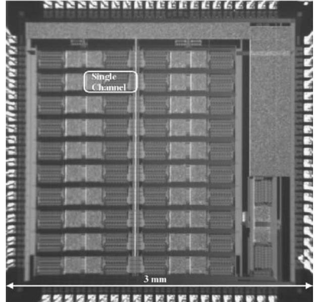
**Fig. 5.** Micrograph of the multi-channel potentiostat interface
