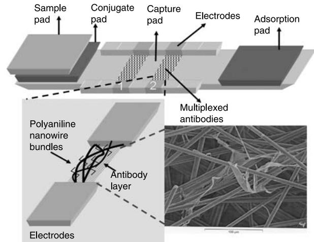
**Fig. 1.** The architecture of the proposed biosensor and a SEM image of the capture pad
