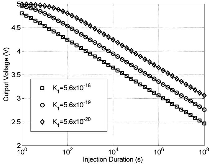
Fig. 7. Response of the floating-gate injector for different values of  $K_1$ .
