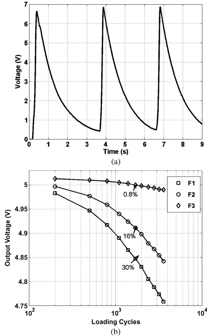
Fig. 13. (a) Voltage generated by a PZT in response to periodic loading. (b) Measured response of the floating-gate injector array.
