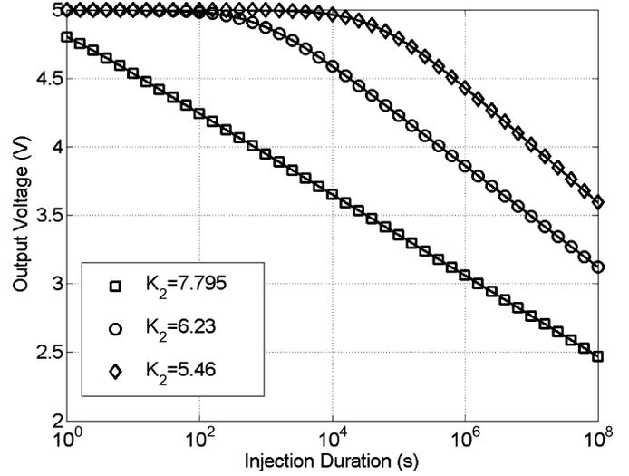
Fig. 6. Response of the floating-gate injector for different values of  $K_2$ .
