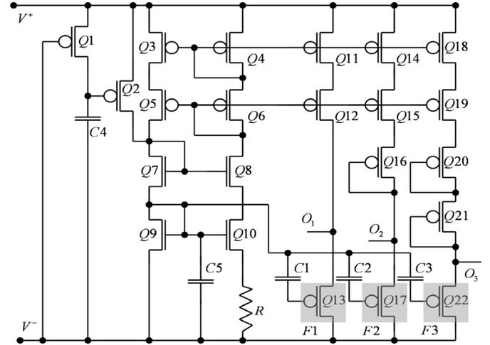
Fig. 8. Circuit implementation of the floating-gate reference array.
