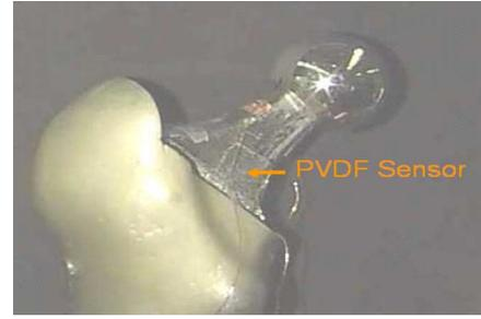
Fig. 2. Stainless steel hip implant reported by the authors in [11] showing PVDF sensor/generator attached for monitoring torsional loading.
