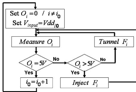
Fig. 10. Flowchart describing the sensor initialization algorithm.
