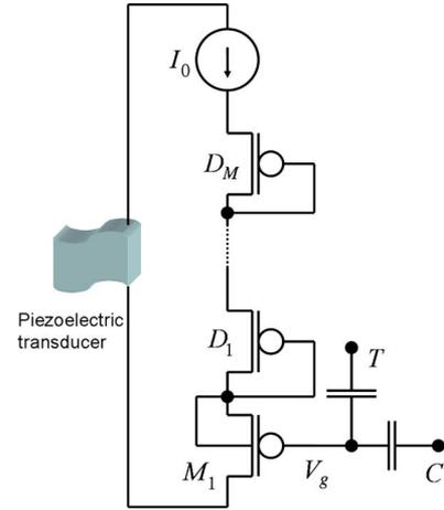
Fig. 4. Simplified circuit model for piezo-driven floating-gate sensor.
