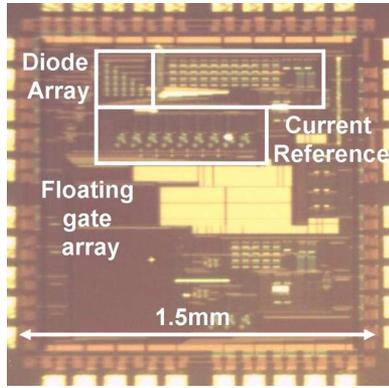
Fig. 9. Micrograph of the prototype floating-gate sensor.
