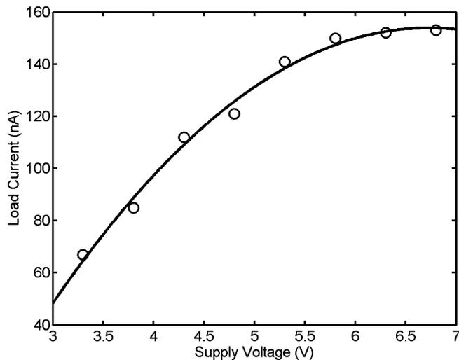
Fig. 14. Supply current drawn by the sensor at different supply voltages.
