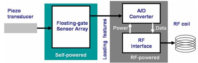
Fig. 15. System architecture of a complete implanted device that integrates the proposed floating-gate sensor array.
