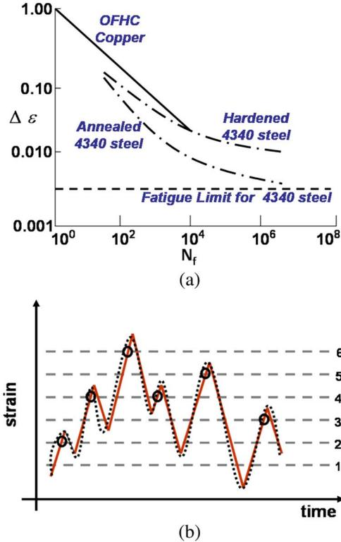
Fig. 3. (a) An example of an S-N curve (redrawn with parameters adapted from [25]). (b) Illustration of the Miner's rule applied to a recorded strain waveform.
